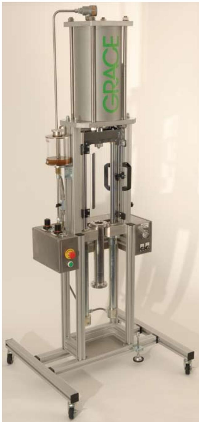
The 1" and 2" MODcol® MultiPacker® instrument is able to pack 25mm i.d. (1") and 50mm i.d. (2") Spring® columns with high performance. The packer has a high safety standard, and can be used in explosion-hazard areas. The ease of use results in reproducible column packing, nearly operator independent. This makes the MODcol® MultiPacker® instrument the ideal choice for column self packing needs in the pharmaceutical industry.
