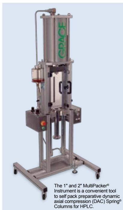
The 1" and 2" MultiPacker® Instrument is a convenient tool to self pack preparative dynamic axial compression (DAC) Spring® Columns for HPLC.
