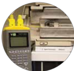
Measure column compartment temperature with the supplied VKIT-1516 probes
