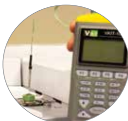
Measure GC inlet temperature with the VKIT-1517 inlet probe
