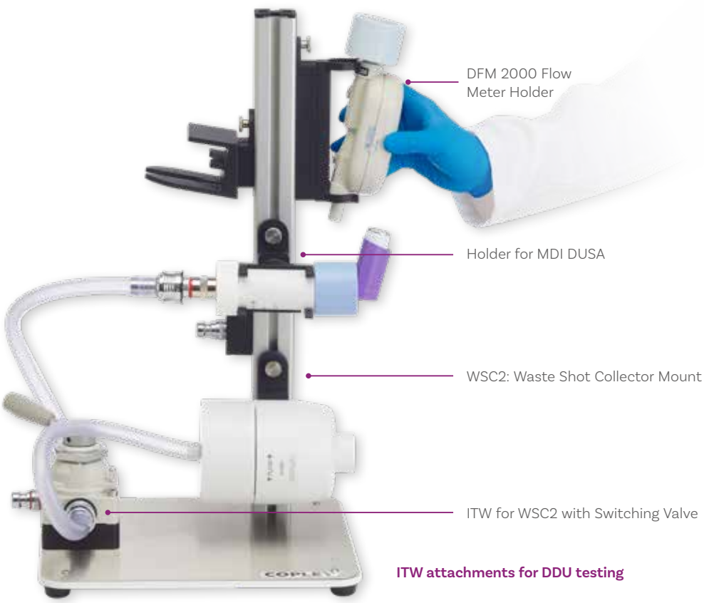
Rotatable DUSA holder enables easy manipulation of the sampling apparatus
